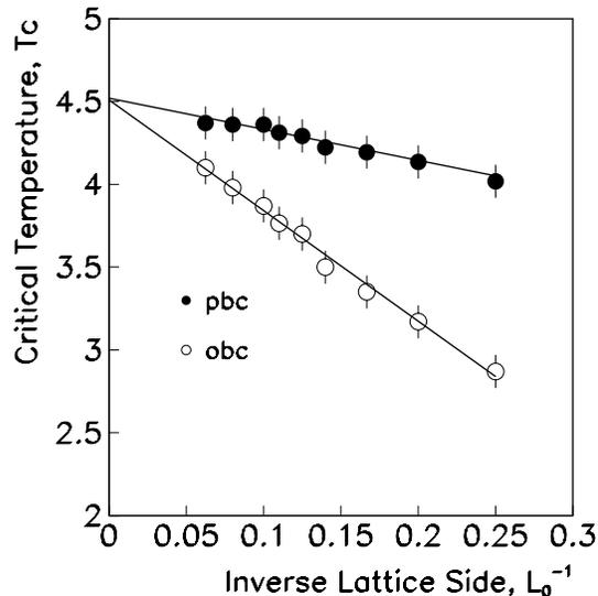
Figure 2: Finite size scaling of the critical temperature of the 3D-Ising model, for lattices of different sizes ( $L_0=4-10,12,16$ ). Dots: results for lattices with periodic boundary conditions. Circles: results for lattices with open boundary conditions. Lines: straight line fits.
