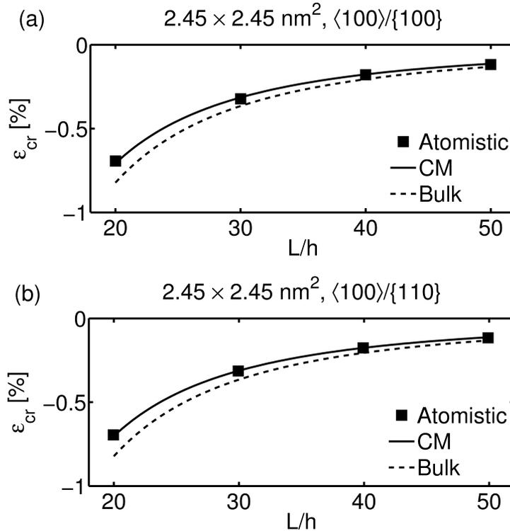
Figure 2. Critical buckling strain for (a)  $\langle 100 \rangle / \{ 100 \}$  and (b)  $\langle 100 \rangle / \{ 110 \}$  nanowires with  $2.45 \times 2.45 \text{ nm}^2$  cross sections for different aspect ratios.
