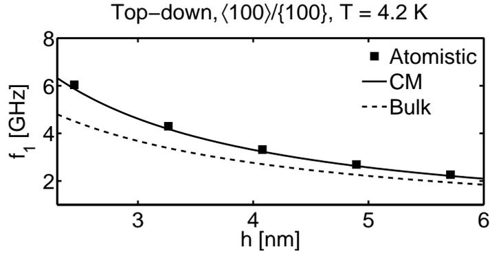
Figure 1. The fundamental eigenfrequency for  $\langle 100 \rangle / \{ 100 \}$  top-down nanowires of different cross sectional dimensions. The aspect ratio of all nanowires is 12. The markers correspond to atomistic results, the solid and dashed lines are predictions from the newly derived continuum model and macroscopic beam theory, respectively.
