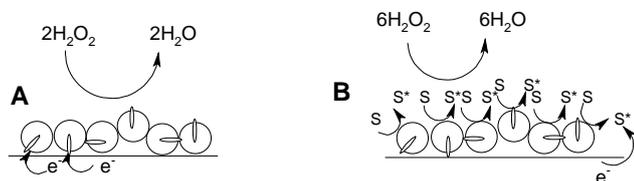
FIG. 1 SCHEMATIC REPRESENTATION OF DIRECT (A) AND MEDIATED (B) ELECTRON TRANSFER IN THE CASE OF PEROXIDASE-GRAPHITE ELECTRODES ILLUSTRATING THE STATEMENT THAT ONLY A PART OF THE IMMOBILIZED PEROXIDASE MOLECULES CAN ACCEPT ELECTRONS DIRECTLY FROM THE ELECTRODE, IN CONTRAST TO DIFFUSING SUBSTRATE RADICALS (S<sup>•</sup>)
