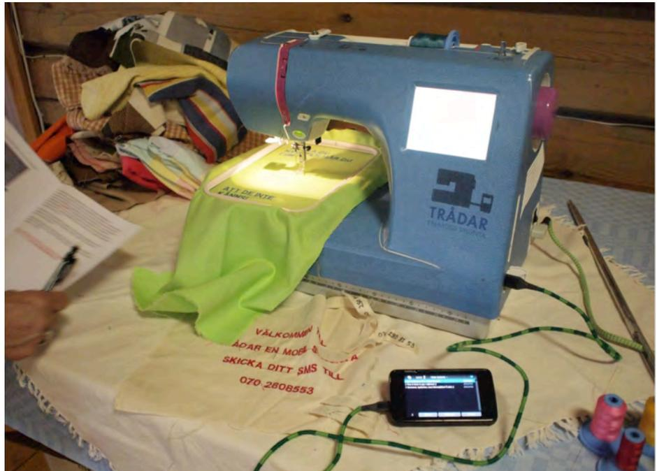
Figure 3. A mobile phone with bespoke software for translating SMS to a specific file format and transferring it to the embroidery machine. Assembled in Gafsele, 2011.
