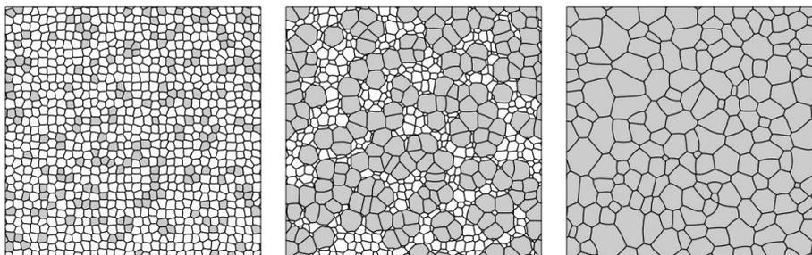
Figure 1: Abnormal growth, from left to right, of (001) grains (gray) at the expense of the (111) texture component (white). The abnormal growth of (001) grains is triggered by a lower stored energy content in this texture component.
