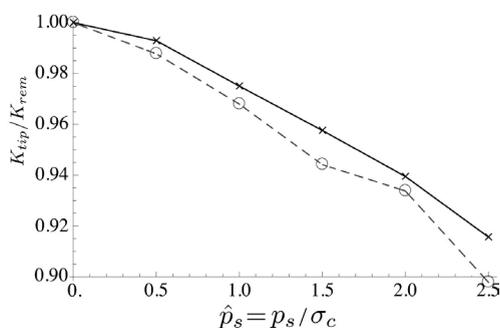
Fig. 4 The relative stress intensity factor  $\hat{p}_s = p_s/\sigma_c$  for isotropic (solid) and anisotropic (dashed) materials
