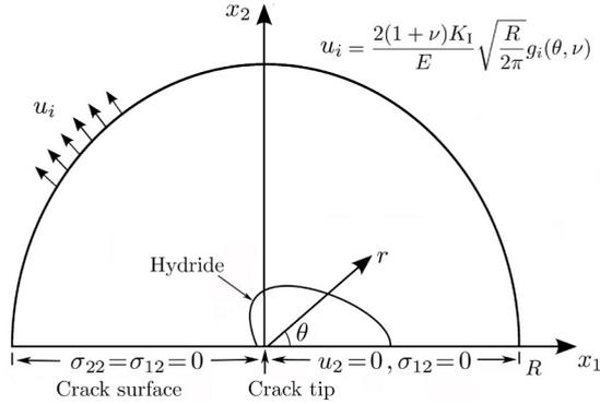
Fig. 1. Semi-infinite crack, near crack tip precipitate zone under remote mode I loading. The boundary conditions are prescribed displacements on the half circular contour, traction free crack surfaces and symmetry conditions in the crack plane ahead of the crack tip.
