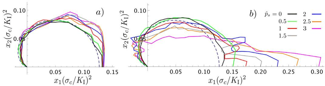
Fig. 2. The shape of precipitates for a) the isotropic ( $q = 0$ ) and b) the anisotropic case with anisotropy factor  $q = 0.16$ , for different dilatation free pressure  $\hat{p}_s$ . The dashed curve is the exact result for  $\hat{p}_s = 0$ .
