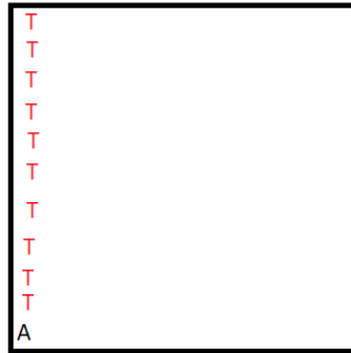
Figur 10: Map of the tested area (A represents the anchor location and the Ts represent the tested tag locations).
