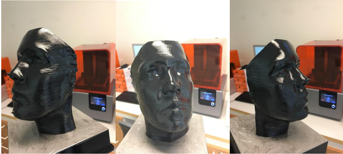
Picture 2: object produced by 3D printing a scan of one of the authors head and then used for the scanning sessions. Measuring points shown between the eyes ( n ), on the tip of the nose ( prn ), the chin ( pg ), left tragus ( trs ) and right tragus ( trd ).
